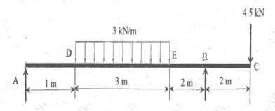
(b) For the beam loaded as shown in figure draw the Shear force and bending 10 moment diagram.
