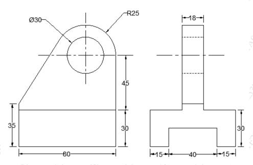
Q.3 (a) The pictorial view of a machine part is shown in following figure.
