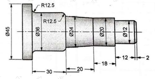
**b** Write a CNC part program using G and M codes for contouring a component as shown in following figure having thickness 5mm. Assume cutter speed as 15m/min and feed rate as 0.2 mm/rev. Assume suitable data if needed.
