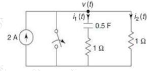
E Find the transmission parameter for the network shown.
