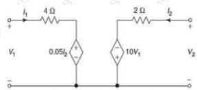
B For the Network shown, write down the f-cutset matrix and obtain the Network equilibrium equation in matrix form using KCL.
