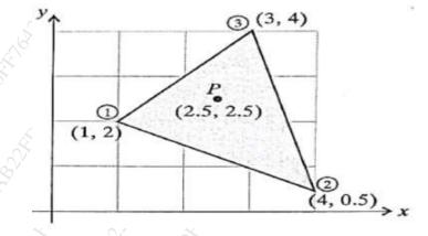
Q5 a) For 2D loaded plat shown in below figure below. Determine the displacements of nodes 1 and 2 and the element stresses using the plane stress conditions. Assume thickness as 10 mm, E = 225 GPa and poisons ratio = 0.25, All Dim are in mm [12]
