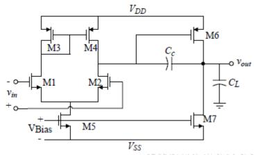
Av > 3000V/V  $V_{DD} = 2.5V$   $V_{SS} = -2.5V$
