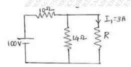
(f) Find the current through  $4\Omega$  resistor by source transformation in the following circuit;
